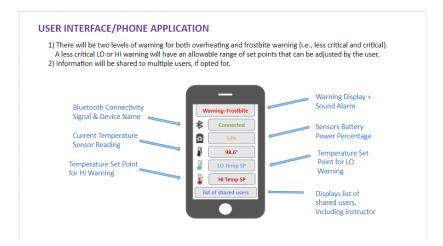
The software side of things consists of two main portions, user interface and logic. On the logic side of things, the main focus is paying attention to the proper parameters ie. temperature and making sure we can warn the people if their body temperature is getting to a dangerous level. From there,
